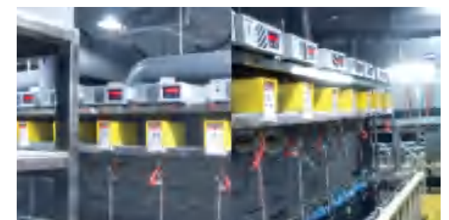
Metal Plating Synchronous power supply 300A/12V
